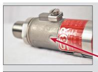
The 815PT and 815DT can be easily configured externally with a magnet. Simply place a magnet to the targets located on the housing for 3 seconds and set the zero and span.
